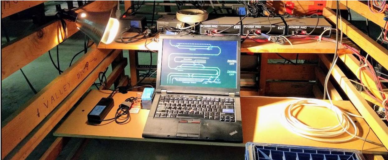
The computer is locked in a dock which provides power and USB connections. The dock itself is secured by a cable lock.
