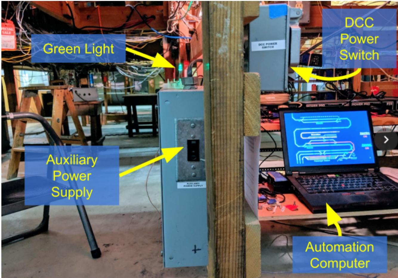
The “Auxiliary Power Supply” is a gray box mounted vertically on the other side of the support where the DCC Power Switch is located. On top of the Auxiliary Power Supply is a green light.
